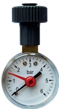
**MABO 50** is a pressure gauge kit expressly designed for pressurizing underfloor systems. Thanks to the 3/4" coupling with free nut, it is compatible with all the fill / drain valves present on the manifolds for radiant systems. It is easily removable and reusable. It's a fundamental tool for every plumber, in compliance with the legislation for testing all radiant heating/cooling systems.
