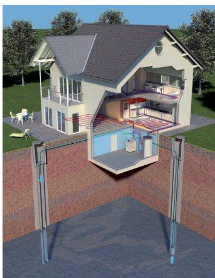
Vertical probes Sonde verticali
